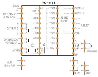
· A1 to A4 : Alarm 1 (A1) to Alarm 4 (A4)
