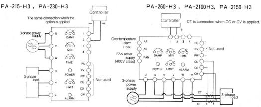
The load can be connected by both Y or A.
